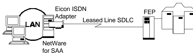
Figure 9: LAN - SNA Connectivity over Leased Lines
